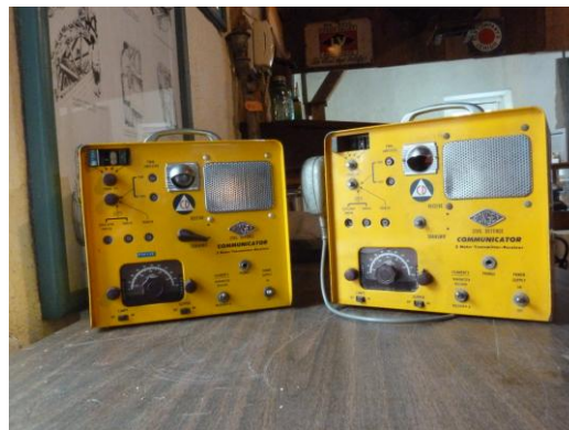
Two Gonset Communicators (circa 1960) discovered in Hellertown Borough Storage. The radios operated on frequencies from 144 to 146 MHz using Amplitude Modulation (AM).
